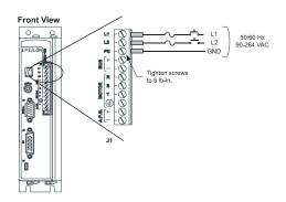
Figure 11: Epsilon AC Power Wiring Diagram
